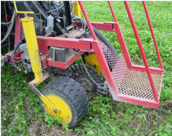
Figure 2. (a.) The waved sampling disc during field testing (b.) the soil analytical and sensing component consists of a mixing chamber, inlets for chemical solutions and water, a pH ISFET sensor and a spinning disc for mixing. Sieved soil is brought into the mixing chamber via a soil measuring unit. The waste outlet from the mixing chamber is controlled using a pinch valve.
