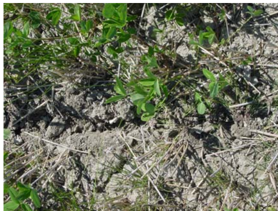
Fig 4. The spinning disc leaves a groove about 20 mm wide. Soil particles not collected by the material fan are also seen beside the groove.
