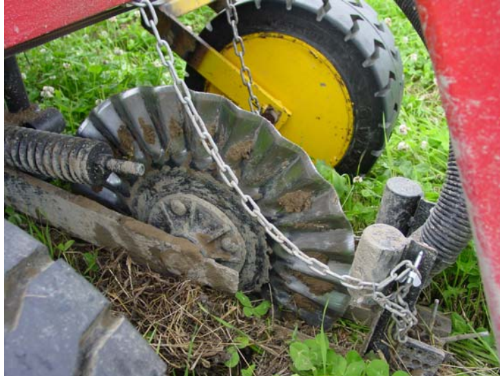
Fig 1. When driving faster than 2 m/s the threaded disc throws up soil, which is collected with a material fan through a tube. The soil passes a cyclone and a rotating sieve before it is analysed in the analytical component.
