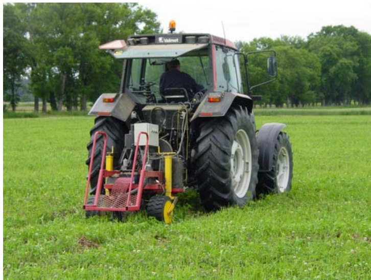
Fig 6. The on-the-go soil sensing system does not operate properly in soils that are wet and have high clay content, i.e. 'sticky muddy' soil
