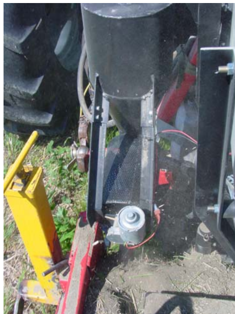
Fig 2. The rotating sieve (seen from above) consists of a cylindrical shaped sieve and a small motor (60 rpm). Larger particles and straw passes through the rotating sieve.
